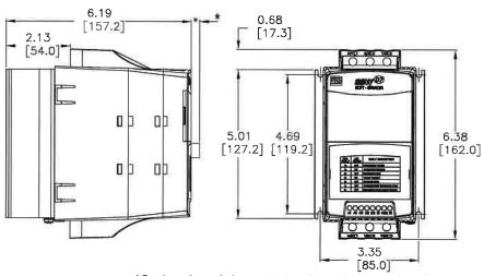
\*Optional modules add depth to dimension as follows: <u>SSW07-08-KRS-485</u> and <u>SSW07-08-KRS-232</u> add 5mm [0.2 in ] <u>SSW07-08-KPTC-MTR</u> adds 5mm [0.2 in ]
